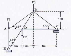
Determine the components of all forces acting on all members of the frame shown. 4(b)
