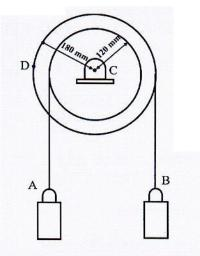
5(b) A drum of radius 90 mm is mounted on a cylinder of radius 120 mm as shown in figure 14 below. A cord is wound around the drum and is pulled in such a way that point D has a velocity 90 mm/s and an acceleration of 450 mm/s<sup>2</sup> both directed to left. Assuming the cylinder rolls without sliding, determine the acceleration of i) of point A and ii) of point C.
