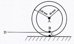
6(a) A homogenous cylinder C and a section of pipe P are in contact (figure shown below) when 15 they are released from rest. Knowing that both the cylinder and the pipe roll without slipping, determine the clear distance between them after 3 sec.
