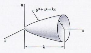
3(b) Determine the moment of inertia of the shaded area shown in the figure below with respect 14 to the Y-axis by direct integration method.
