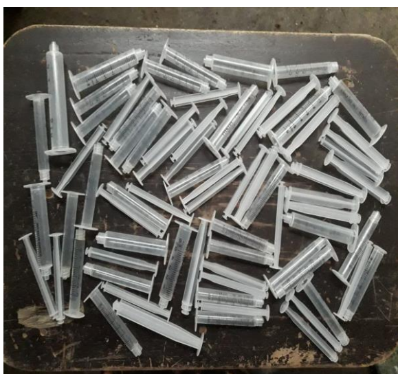
Figure 4.2: Photographic View of Washed and Sun-dried Syringe Waste Materials
