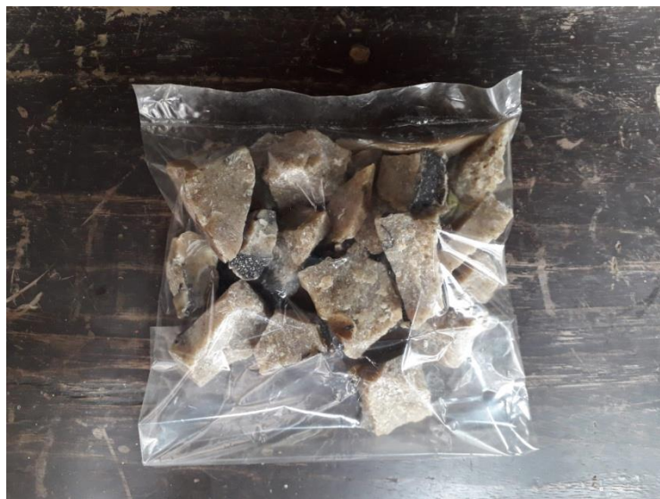
Figure 5.3: Photographic View of Pyrolytic Char Derived from Syringe Waste
