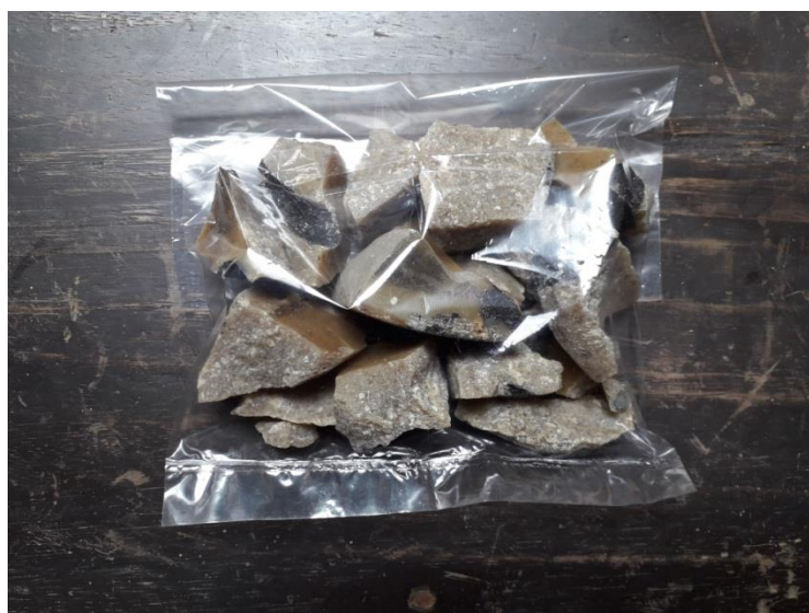
Figure 5.4: Photographic View of Pyrolytic Char Derived from Saline Bottle Waste
