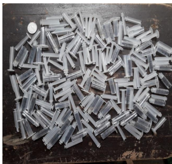
Figure 4.3: Photographic View of Prepared Feed Materials of Syringe Waste for Pyrolysis
