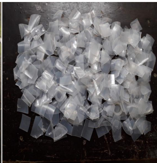
Figure 4.5: Photographic View of Prepared Feed Materials of Saline Bottle Waste for Pyrolysis
