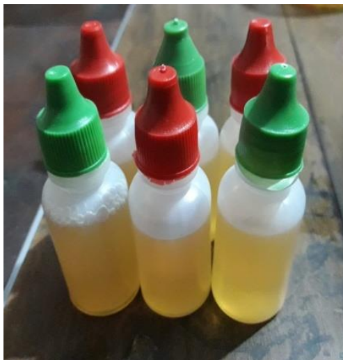
Figure 5.1: Photographic View of Pyrolytic Oil Derived from Syringe Waste
