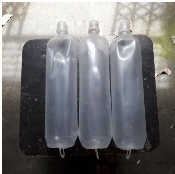
Figure 4.4: Photographic View of Washed and Sun-dried Saline Bottle Waste Materials
