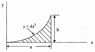
3(b) Determine the moments of inertia  $\bar{l}_x$  and  $\bar{l}_y$  of the area shown with respect to centroidal axes respectively parallel and perpendicular to side AB.
