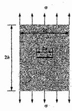
$$k = \sigma \sqrt{\pi a} \left[ \frac{1 - \frac{a}{2b} + 0.326 \left(\frac{a}{b}\right)^2}{\sqrt{1 - \frac{a}{b}}} \right]$$
