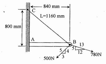
1(c) Two cables are tied together at C and loaded as shown. Knowing that P=500N and  $\alpha$ =60°, determine the tension in (i) cable AC, (ii) cable BC.
