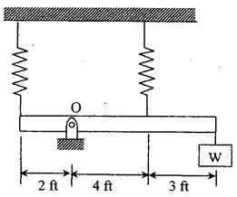
7(a) Write the shear and moment equations and draw the shear force and bending moment diagrams for the beam loaded as shown in the figure.
