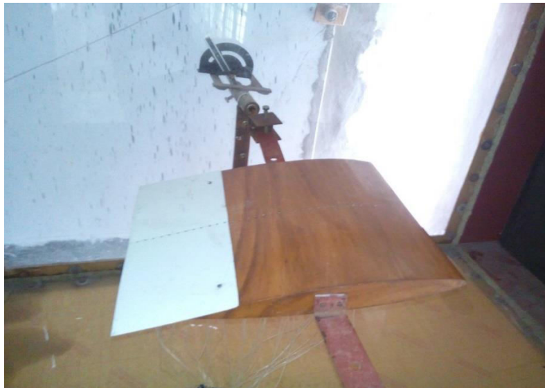
Figure 3.6: Airfoil with extended trailing edge inside wind tunnel
