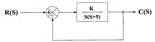
6(c) For the SFG as shown in the figure, find the overall transmittance of the system.
