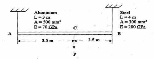
2(c) The rigid bar ABC in figure below is pinned at B and attached to the two vertical rods, the bar is horizontal and the vertical rods are stress free. Determine the stress in the aluminium rod if the temperature of the steel rod is decreased by 40° C. Neglect the weight of the bar ABC
