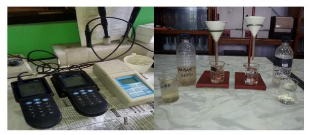
Photo 10: EC, pH and turbidity test
