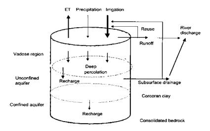
Figure 2.7: Free body diagram of water flows in the San Joaquin Valley
