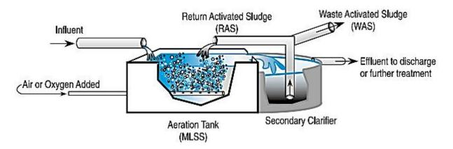
Figure 2.10: Basic schematic of the biological process in an activated sludge processing unit
