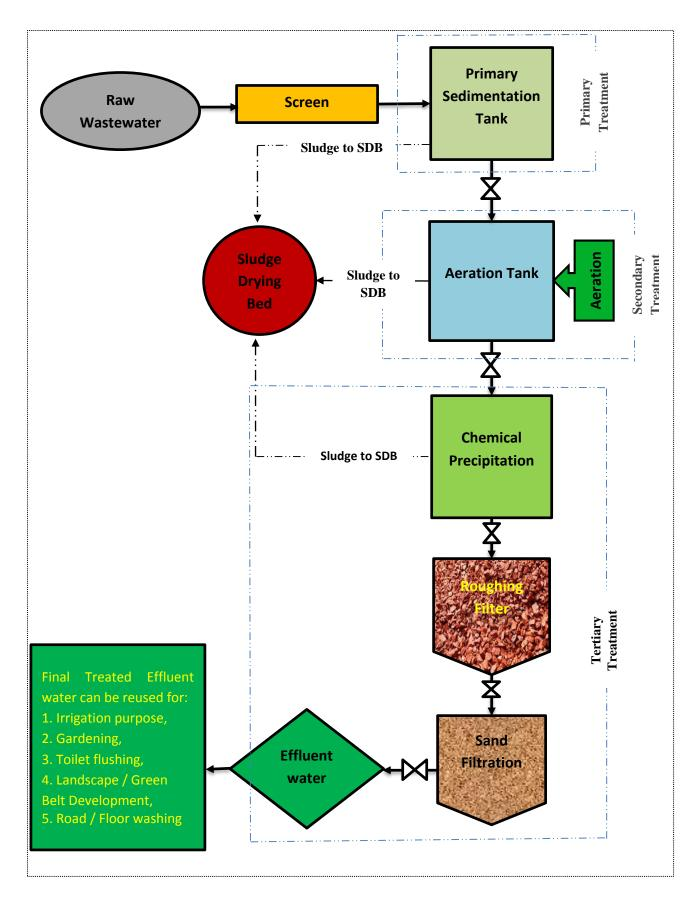
Figure 3.6: Flow diagram showing the proposed laboratory scale treatment units
