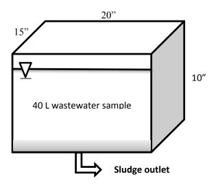
Figure 3.5: Plain sedimentation tank for primary treatment of wastewater
