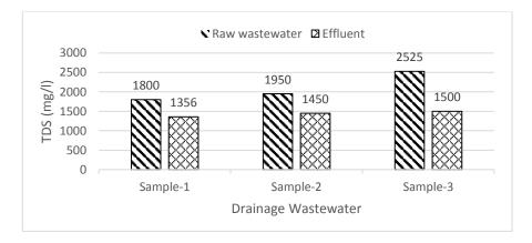
Figure 5.5: TDS concentration of raw and treated wastewater
