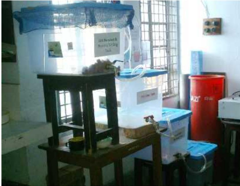
**Figure 3.7** Laboratory setup of treatment unit for market wastewater
