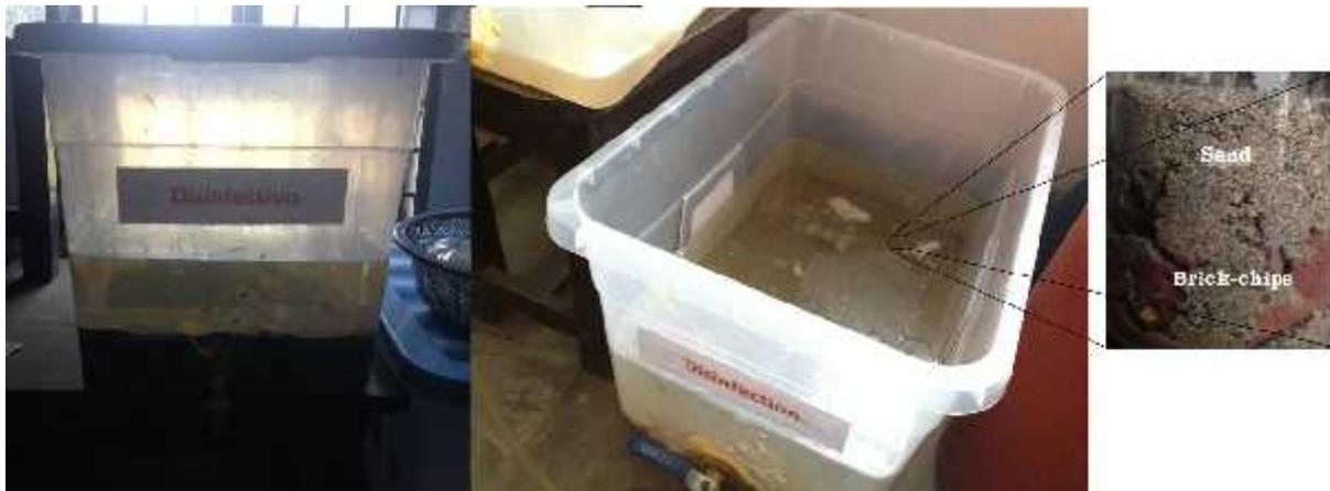
**Figure 5.2** The modified dual-media treatment unit of market wastewater
