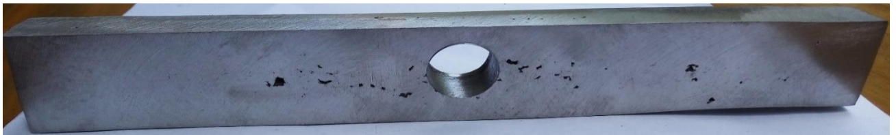
Figure 4.14: Flat bar type mild steel sample.
