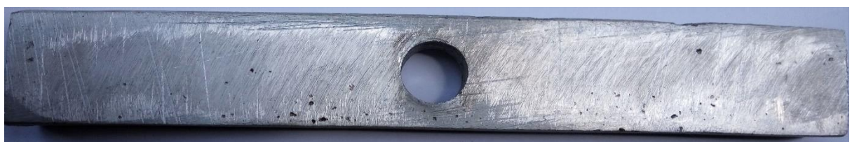
Figure 4.16: Flat bar type cast iron sample.
