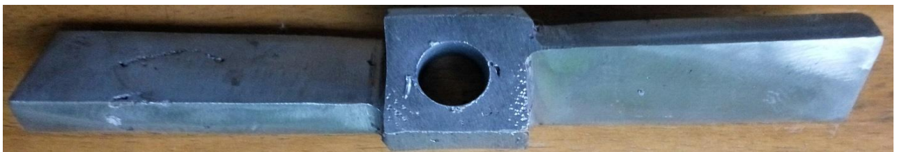
Figure 4.15: Impeller type mild steel sample.
