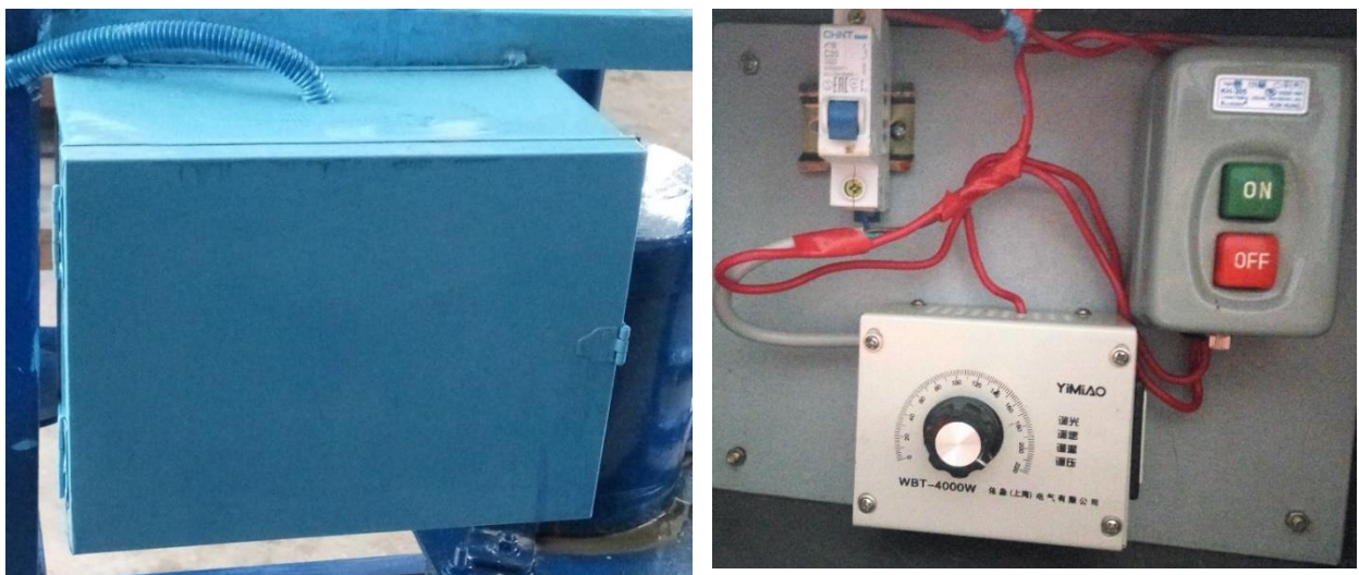
Figure 4.7: Control box of the slurry erosion tester.
