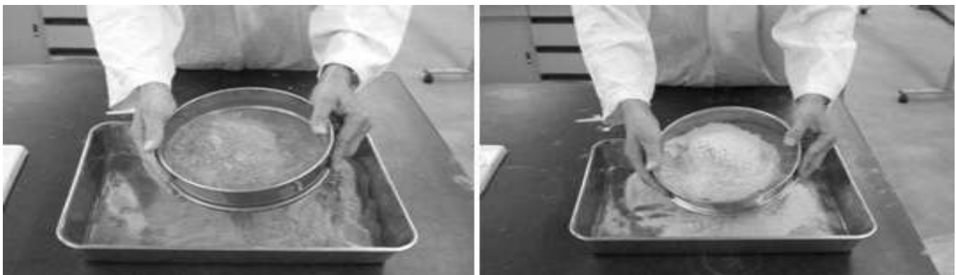
Figure 3.5 Sieve analysis and rice bran
