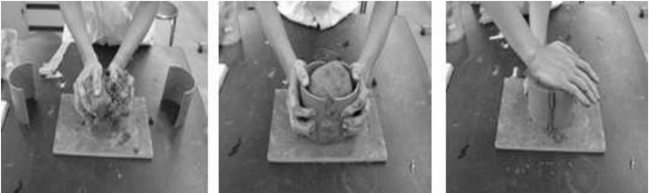
Figure 3.7 Shaping of candle from dough using dice
