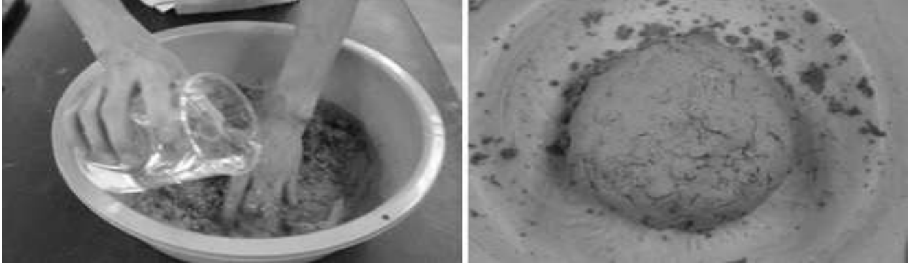
Figure 3.6 Mixing of soil & rice bran and making dough with water
