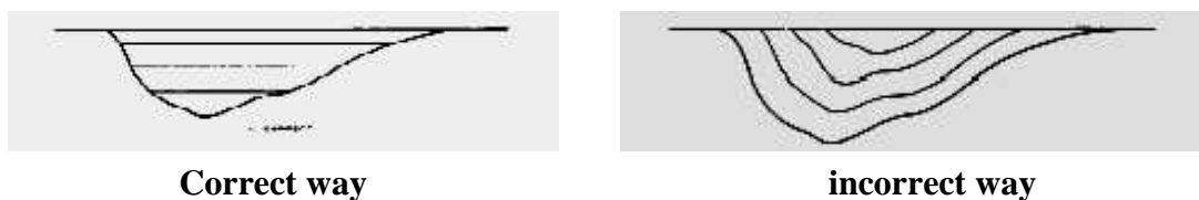
Figure 5.1: Back fill in deep depression
