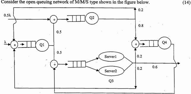
The mean service rates are  $\mu_1 = \mu_3 = \mu$  and  $\mu_2 = \mu_4 = 0.5\mu$ . Externals arrival are at  $Q_1$  and  $Q_2$ following Poisson process.
