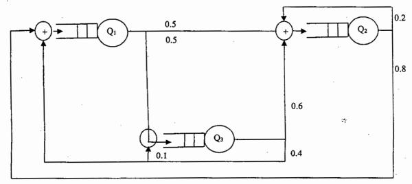
The average service rates of  $Q_1$ ,  $Q_2$  and Q are respectively  $\mu_1 = 1$ ,  $\mu_2 = \mu_3 = 0.5$ . The system has a total user population of 4. Using the convolution approach, obtain the followings:
