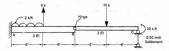
7. Analyze the frame by stiffness matrix method and draw SFD and BMD. Assume (35) reasonable value of El
