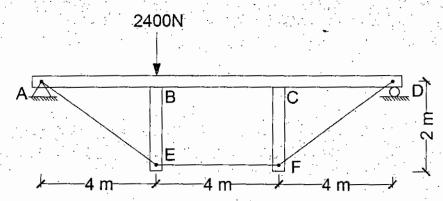
(a) Draw the influence lines for the vertical reaction at A, bending moment at D and (20) share at E of the following beam at a interval of 2 m, where EI is constant.
