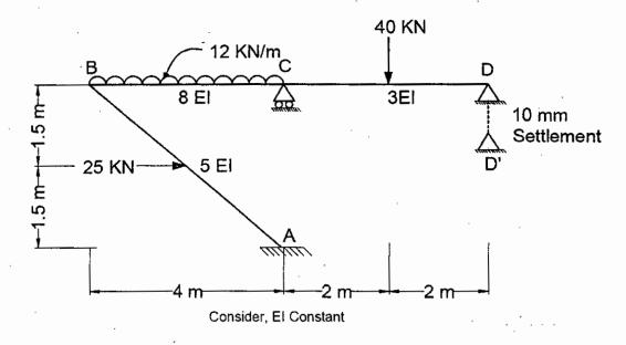
Write down the characteristic of the beam element stiffness matrix. Analyze the (35) beam by stiffness matrix method and draw SFD and BMD. Assume reasonable value of EI.
