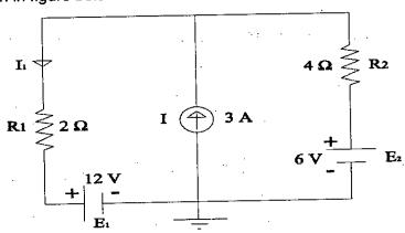
(d) Find the Thevenin equivalent circuit for the electrical network shown in figure (13) below. Use ab as reference.
