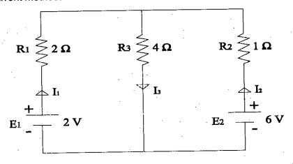
(d) Determine I<sub>1</sub> and I<sub>2</sub> of the figure shown in below using nodal analysis. (10)
