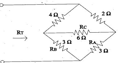
(c) Determine I<sub>1</sub>, I<sub>2</sub> and I<sub>3</sub> of the electrical network of figure shown in below using (10) branch-current method.
