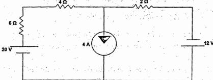
(c) Determine node voltages of figure below. (12)
