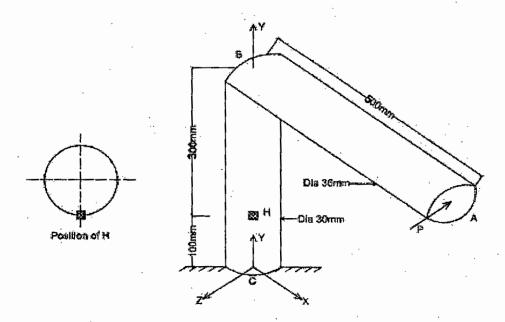
3. (a) Compute the combined stresses at A, B, C and D shown in figure below.
