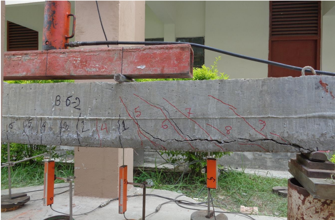
Figure 5.26: Failure mode of beam strengthened with steel bars (B6-2)
