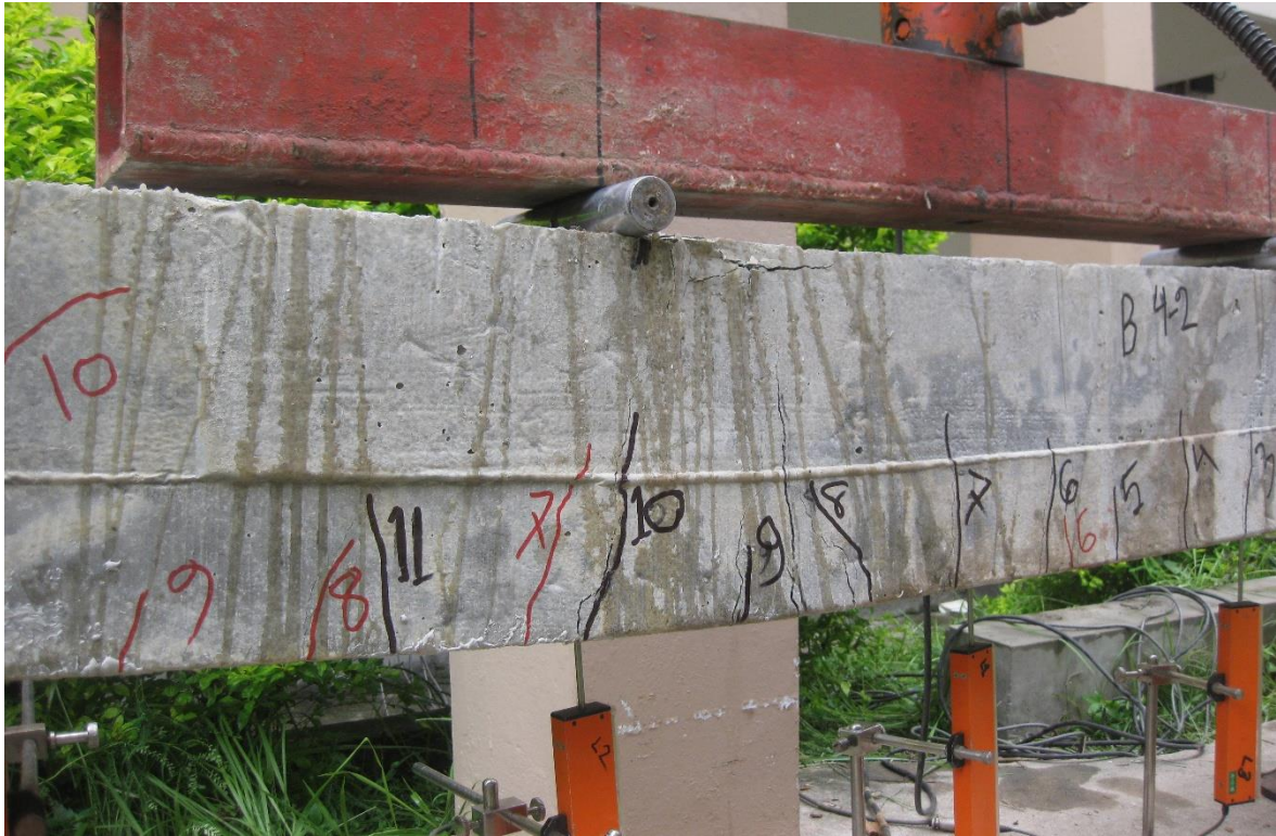
Figure 5.18: Failure mode of beam strengthened with NSM bars (B4-2)
