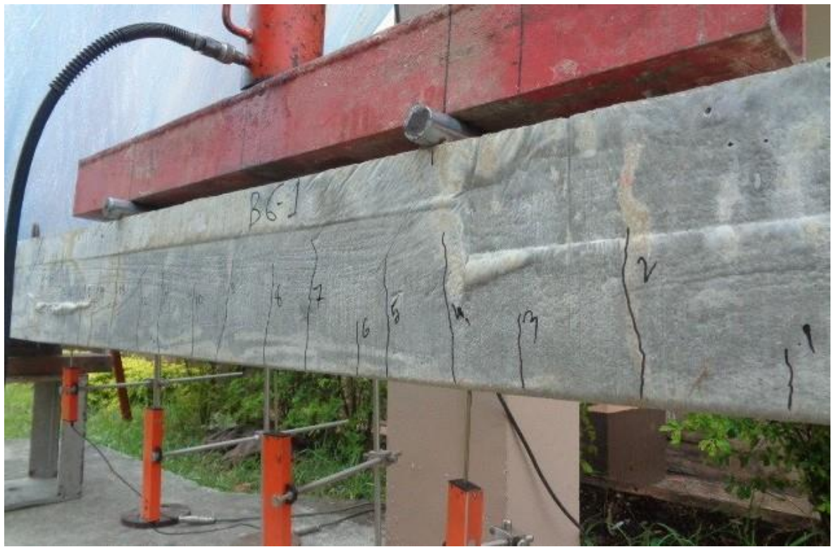
Figure A-18: Crack pattern for preloading (B6-1)
