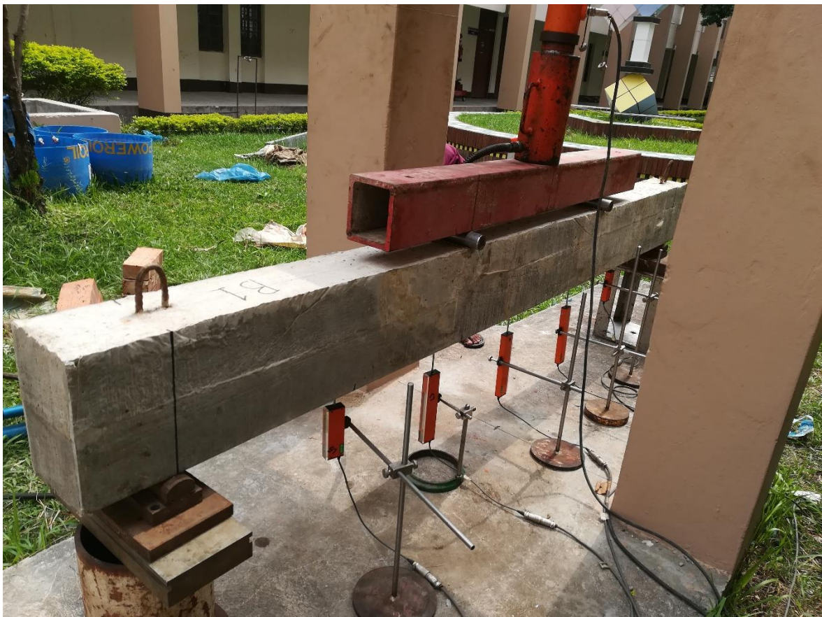
Figure 4.9: Experimental setup for the flexural test
