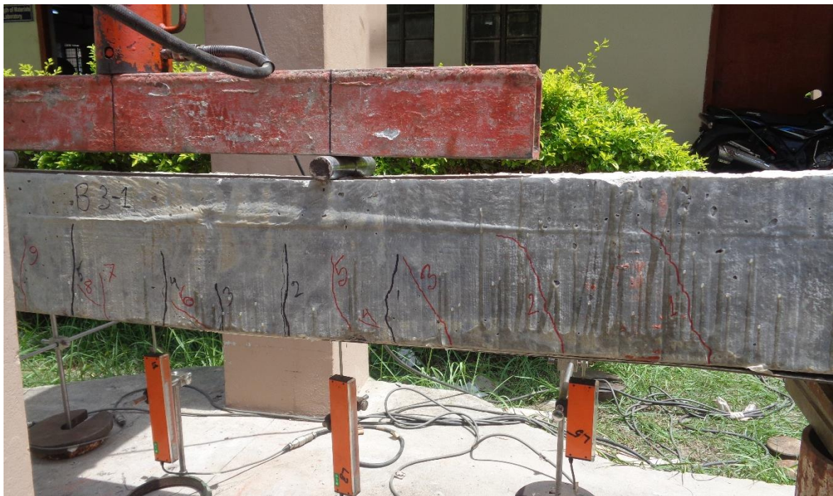
Figure 5.12: Failure mode of beam strengthened with steel plate and bolts (B3-1)
