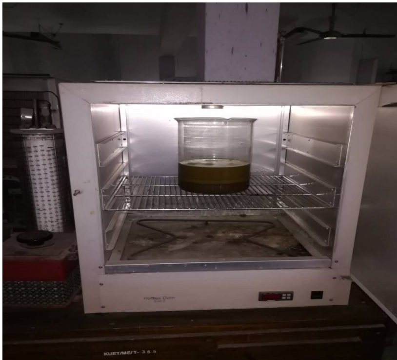
Figure 3.1: Sample Oven Drying and Sterilization at 121°C.
