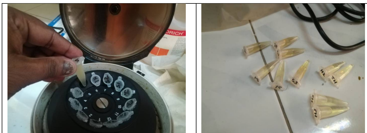
Figure 3.6: Centrifugation of the Experimented Sample Broth
