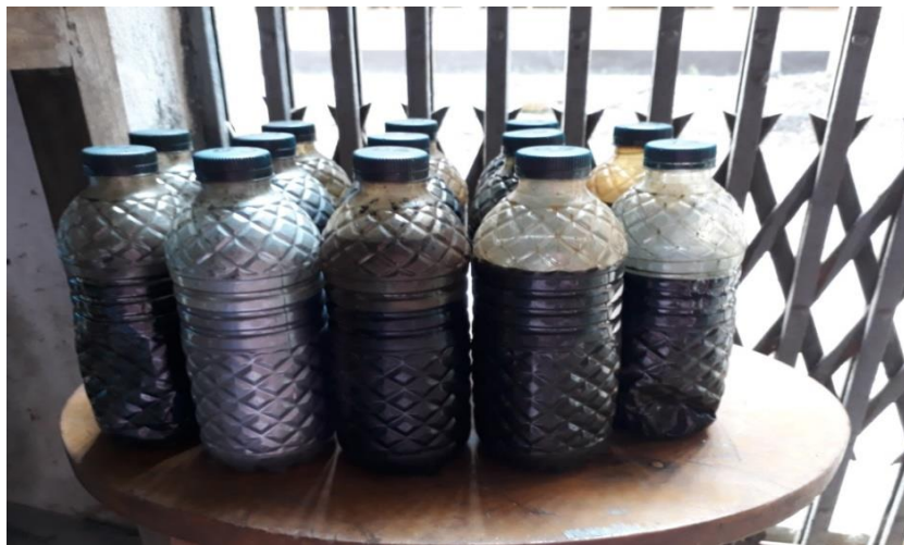
Figure 5.1: Pyrolytic Oil after Production from Shoe/sandal Sole Pyrolysis
