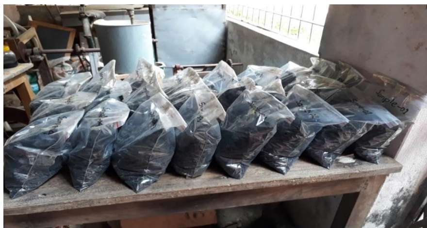
Figure 5.3: Pyrolytic Solid after Production from Shoe/sandal Sole Pyrolysis
