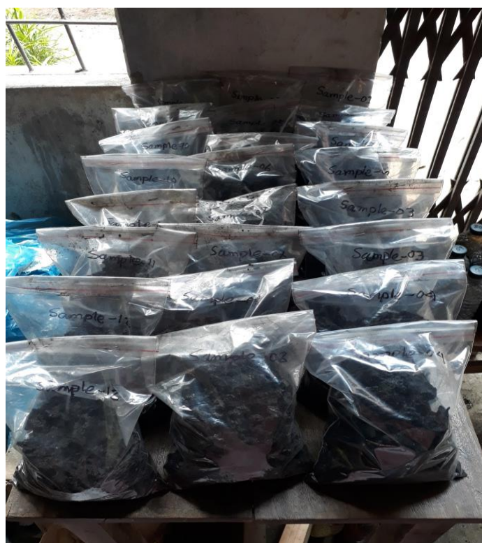
Figure 5.4: Pyrolytic Solid Sample after Production from Shoe/sandal Sole Pyrolysis
