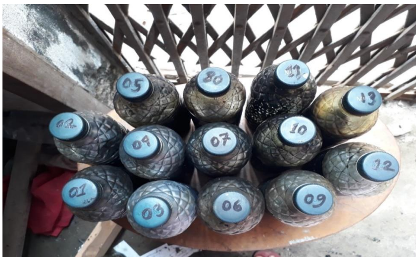
Figure 5.2: Pyrolytic Oil Sample after Production from Shoe/sandal Sole Pyrolysis
