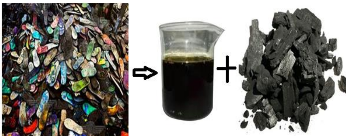
Figure 5.23: Waste Sole of Shoe/sandal is converted to Pyrolysis Oil and Char
