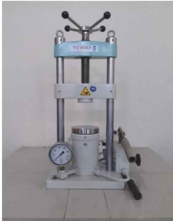
Figure 3.4: Hydraulic press and dies for preparing sample
