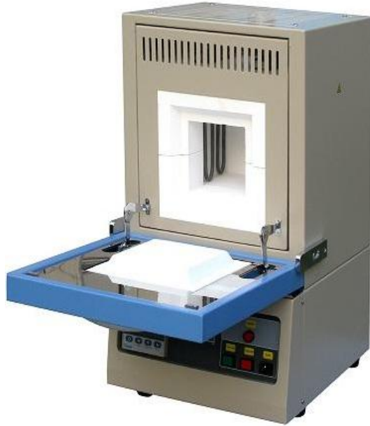
Figure 3.5: High Temperature Muffle Furnace (KSL-1700X-S) at Solid State Physics Lab, KUET.
