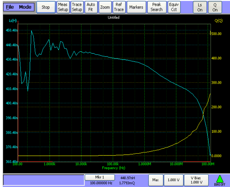
Figure 3.12: Complex permeability measurement by Wayne Kerr Precision Impedance Analyzer
