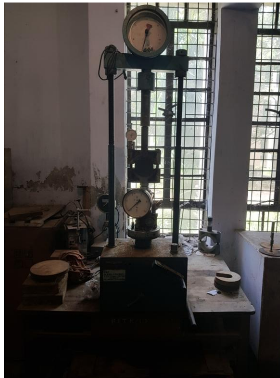
Figure:3.8 Marshall Test Setup
