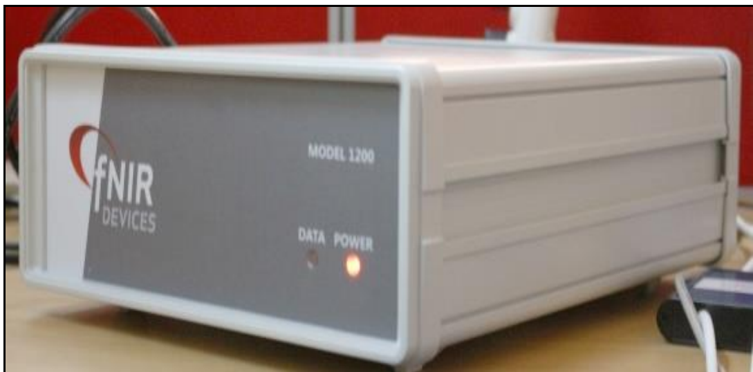
Figure 2.2: A 16 Channel fNIR signal Acquisition device. (Biopac 1200 Model)
