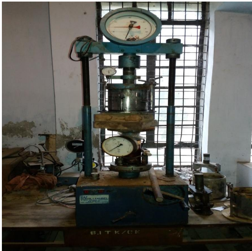
Figure 3.6: CBR testing machine in the laboratory.
