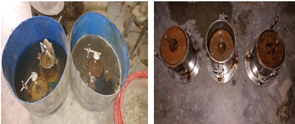
Figure 3.5: Curing and cured sample for CBR test.
