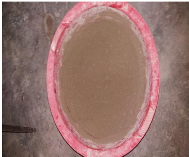
Figure 3.3: Prepared sample for CBR test.
