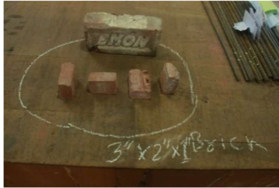
Figure 3.1: Bricks used for infill in the specimen
