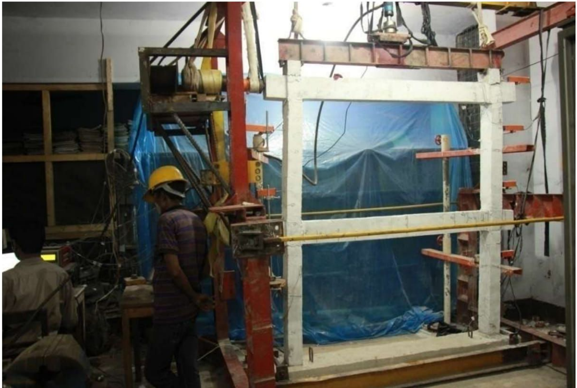
Figure 4.3: Specimen 1, Failure of two storied single bay bare frame
