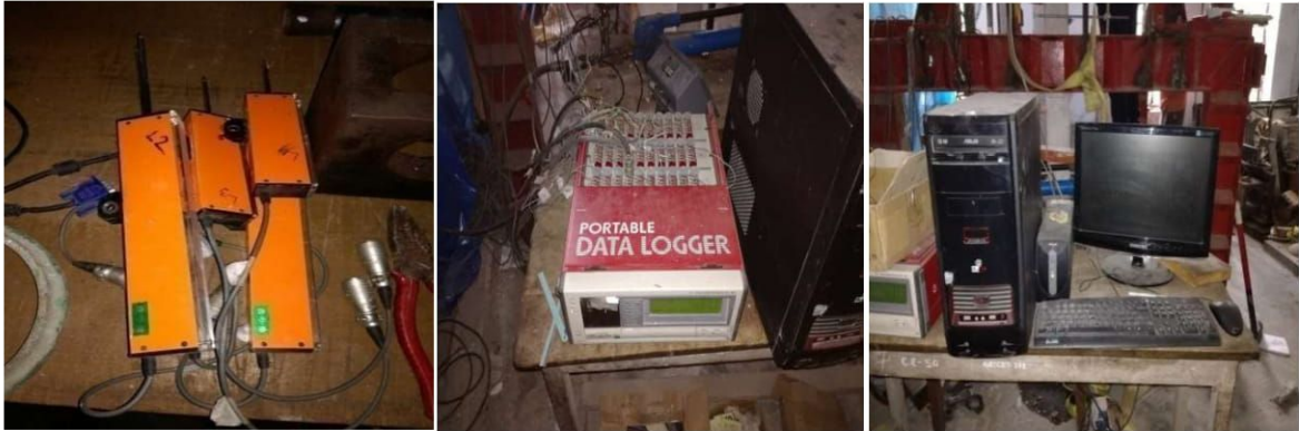
Figure 3.4: LVDTs, data logger and computer set used for testing of specimens
