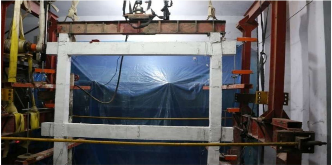
Figure 4.1: Specimen 1, Instrumentation of two storied single bay bare frame
