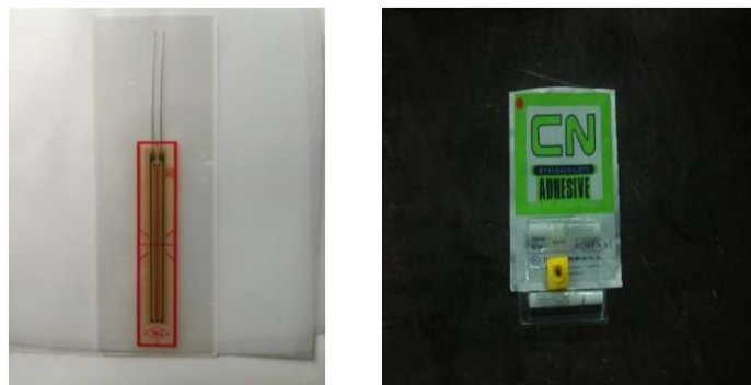
Figure 3.3: Strain gauge, adhesive used on the surface of specimen
