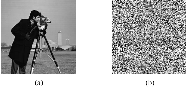
Figure 2.16: Scrambling image using game of life cellular automata: (a) cameraman image, (b) Scrambled image after 5 th generation of GOL.
