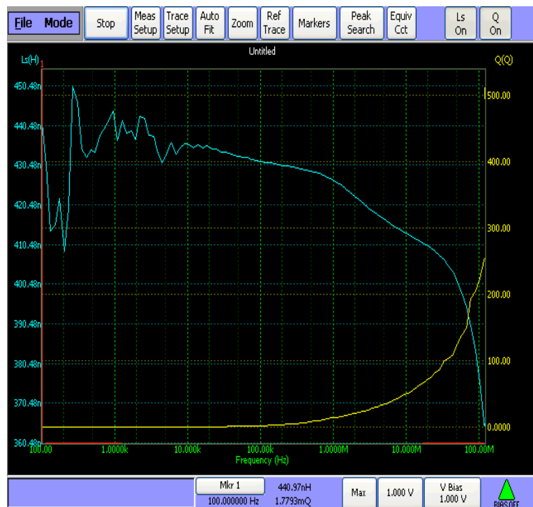
Figure 3.11: Complex permeability measurement by Wayne Kerr Precision Impedance analyzer
