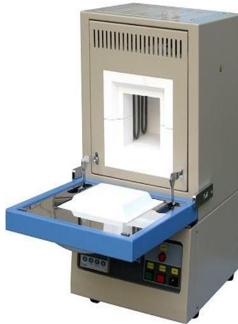
Figure 3.4: High Temperature Muffle Furnace (KSL-1700X-S) at Solid State Physics Lab, KUET
