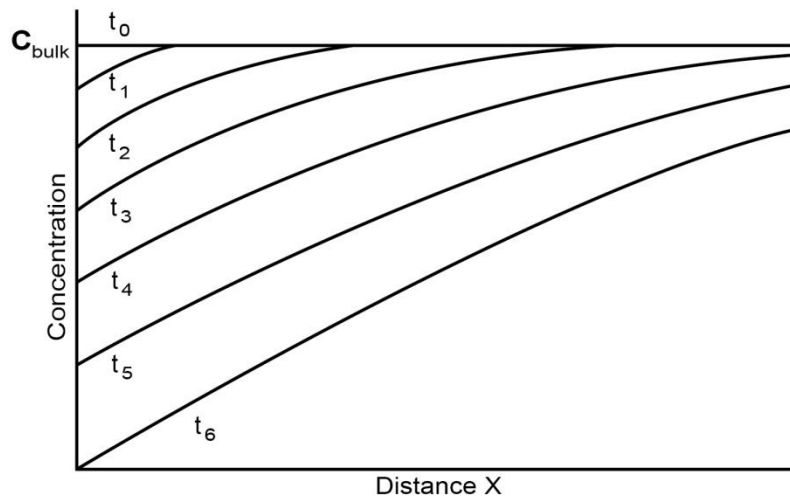
Figure 1.09: Concentration profiles extending into bulk solution during constant-current depletion of species at electrode surface, t_6 > t_0 [87]
