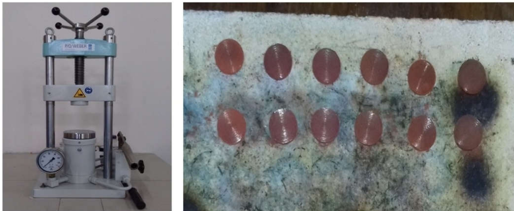
Figure 3.5: Hydraulic press in solid-state lab of KUET and the prepared samples
