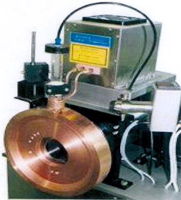
Fig. 2.8 Thin layer of molten alloy intimate contact with the outer surface of metallic rotor is quenched in to amorphous
