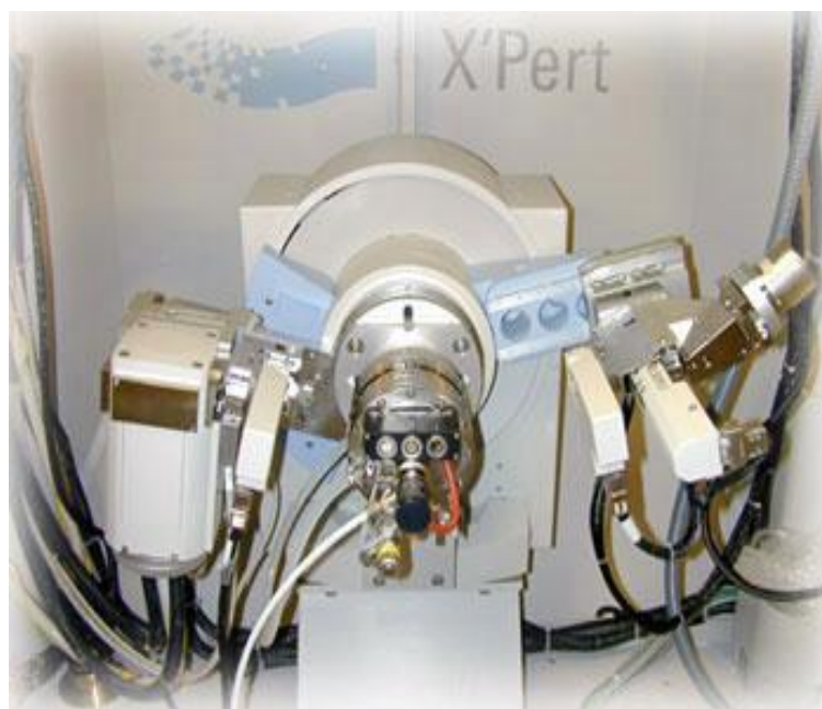
Figure 3.8: Internal arrangement of a PHILIPS X' Pert PRO X-ray diffractometer
