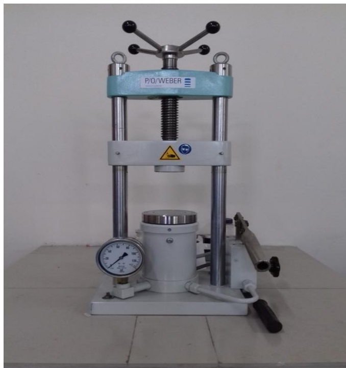
Figure 3.2: Hydraulic press used to make different shaped samples
