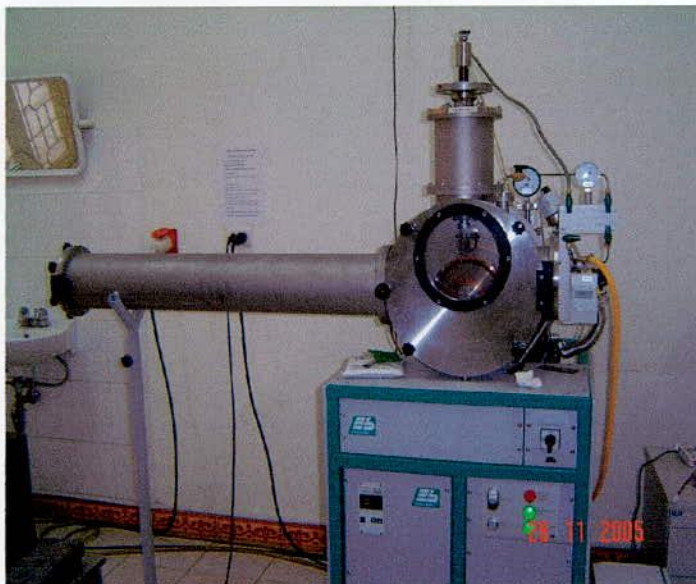
Fig. 3.1 Vacuum arc Melting Machine
