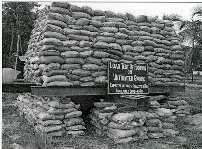
Figure 4.12 Set up of load arrangement for footing load test.
