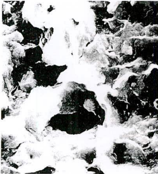
Figure 2.8(a) REM image of kaolinitic clay, scale 5000x. High non-communicating microporosity, electrically neutral two-layer mineral without swelling potential. Preferable mineral phase for cap liners.
