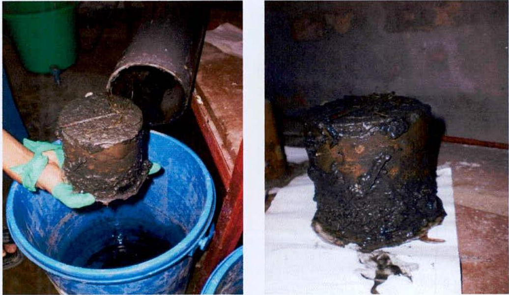
Fig: 3-5 Formation of cake layer on some portion of the membrane surface
