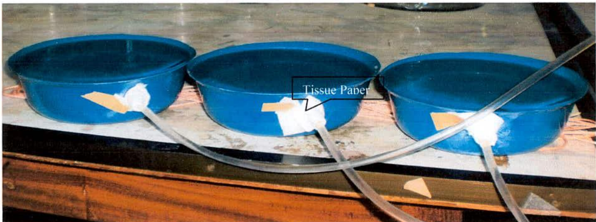
Figure 3.5.1: Water tightness testing arrangement of Upper bucket in the laboratory engineering laboratory, KUET. After setting up the overflow pipe with the upper pot, a tissue paper has been tied up with the periphery of the pipe at outer side of the pot from where leakage can be identified. Then the pot has been made full up to its top with tap water and kept for several hours. The tissue paper has been checked and confirmed its dryness. The Figure 3.5.1 shows the water tightness testing for upper pot.
