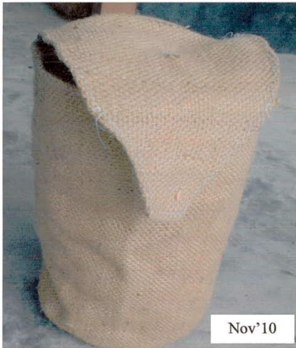
Figure 4.5.5: Textile cover (Jute fiber) before installation (Nov'10)
