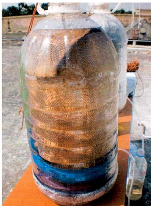
Figure 3.5.2: Water Tightness Testing of Joint Figure 3.5.3: Leakage of Joint
