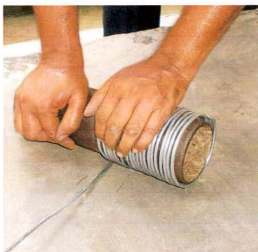
Figure 3.3.1: Making of aluminum wire frame Figure 3.3.2: Aluminum wire flexible frame
