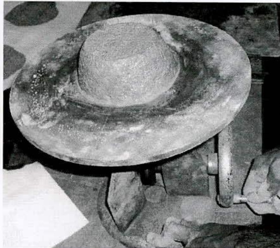
Figure 3.9: Photograph of flow table test arrangement for mortar sample
