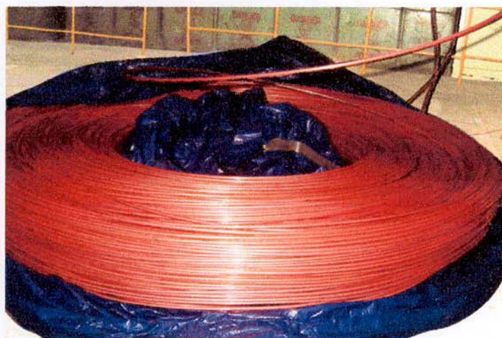
Figure-3.2-1: Copper rod the main and costly raw material of BCSL.
