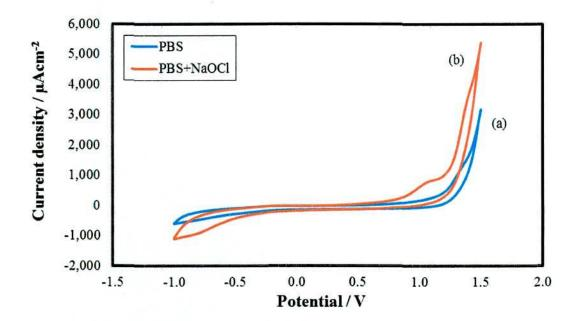
Figure 4.5(a): CVs in 2B PGE (a) in the absence of NaOCl and (b) in the presence of 10 mM NaOCl in 0.1M PBS at E<sub>app</sub>=1.5V (scan rate: 0.05 V/s).
