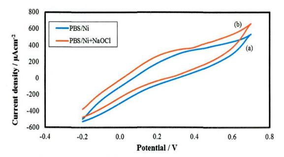
Figure 4.10: CVs of 0.1 M PBS ZnO/PGE (a) without NaOCl (b) in the presence of NaOCl at  $E_{app}$ = 0.7 V (scan rate: 0.05 V/s).
