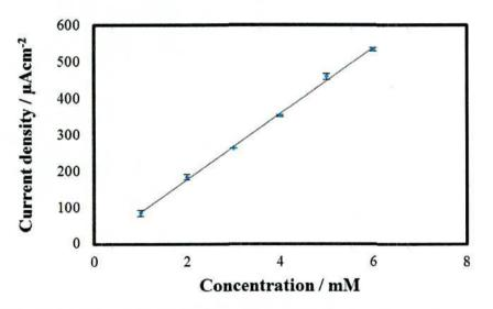
Figure 4.12: The plot of concentration effect current density vs the corresponding concentrations of NaOCl in PGE.
