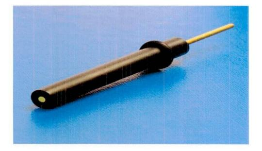
Figure 1.7: GC disk working electrode.
