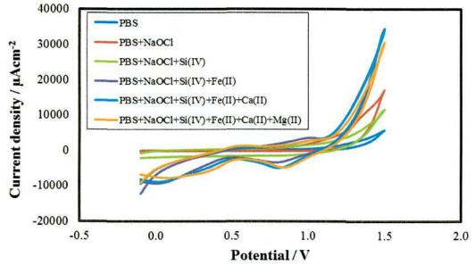
Figure 4.15: CVs in 2B PGE (a) in the absence of NaOCl (b) in the presence of 10mM NaOCl (c) added SiO<sub>2</sub>, FeCl<sub>2</sub>, Ca(NO<sub>3</sub>)<sub>2</sub> and Mg(NO<sub>3</sub>)<sub>2</sub> in 0.1M PBS containing at E<sub>app</sub>= -0.1 to 1.5V (scan rate: 0.05 V/s).
