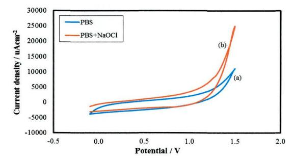
Figure 4.13: CVs in 2B PGE (a) in the absence of NaOCl and (b) in the presence of 10 mM NaOCl in 0.1M PBS at E<sub>app</sub>=1.5V (scan rate: 0.05 V/s).
