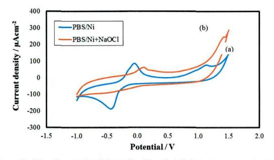
Figure 4.9: CVs of 0.1 M PBS NiO/PGE (a) without NaOCl (b) in the presence of NaOCl at  $E_{app}$ = 1.5 V (scan rate: 0.05 V/s).
