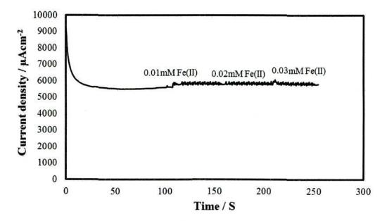
Figure 4.18: Typical amperometric current response of the 2B PGE upon the successive injection of FeCl<sub>2</sub> at E<sub>app</sub>=1.5 V 0.1 M PBS pH 7.
