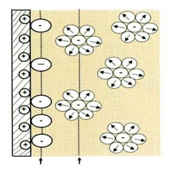
Figure 1.5: Schematic representation of the electrical double layer [76].
