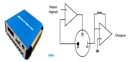
Figure 1.10: A potentiostat with circuit diagram of a three-electrode system.
