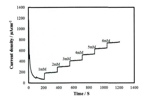
Figure 4.11: Typical amperometric current response of the 2B PGE upon the successive injection of NaOCl with concentrations from 1 mM to 6 mM into a stirred at  $E_{app}$ =1.5V in 0.1 M PBS pH 7.
