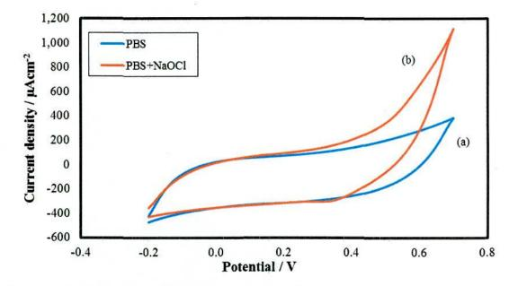
Figure 4.5(b): CVs in 2B PGE (a) in the absence of NaOCl and (b) in the presence of 10 mM NaOCl in 0.1M PBS at  $E_{app} = 0.7V$  (scan rate: 0.05 V/s).
