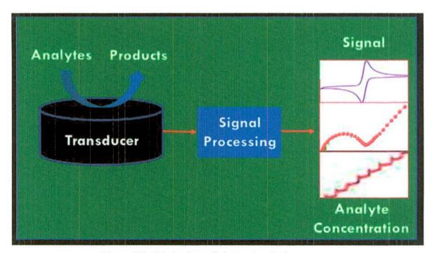
Figure 1.3: Mechanism of electrochemical sensor.
