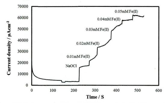
Figure 4.16: Typical amperometric current response of the 2B PGE upon the successive injection of  $1^{st}$  NaOCl and other step FeCl<sub>2</sub> into at  $E_{app}=1.5$ V in 0.1 M PBS pH 7.
