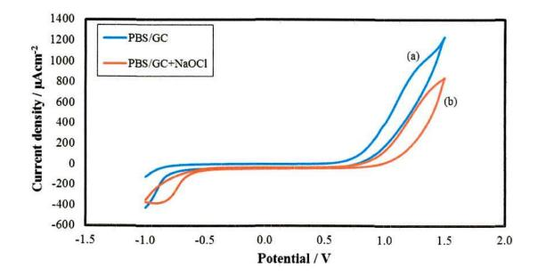
Figure 4.4: CVs in bare GC electrode (a) in the absence of NaOCl and (b) in the presence of 10 mM NaOCl; in 0.1M PBS at E<sub>app</sub>=1.5V (scan rate: 0.05 V/s).
