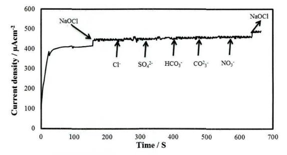
Figure 4.22: Interference test of the sensor in 0.1 M PBS at 1.5V with NaOCl and other interferents including 0.0018, 0.0135, 0.0113, 0.0145 and 0.0073 mM chloride ion, sulfate ion, bicarbonate ion, carbonate ion, and nitrate ion.
