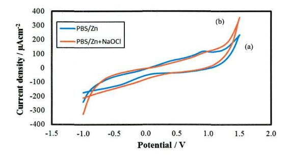
Figure 4.8: CVs of 0.1 M PBS ZnO/PGE (a) without NaOCl (b) in the presence of NaOCl at  $E_{app}$ = 1.5 V (scan rate: 0.05 V/s).
