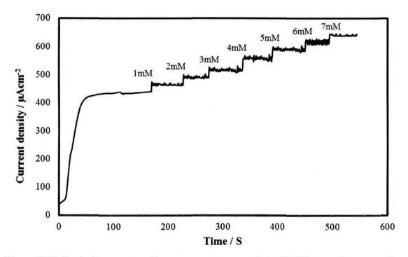
Figure 4.20: Typical amperometric current response of the PDPE upon the successive injection of NaOCl with concentrations from 1 mM to 7 mM into stirred at  $E_{app}$ = 1.5V 0.1 M PBS pH 7.
