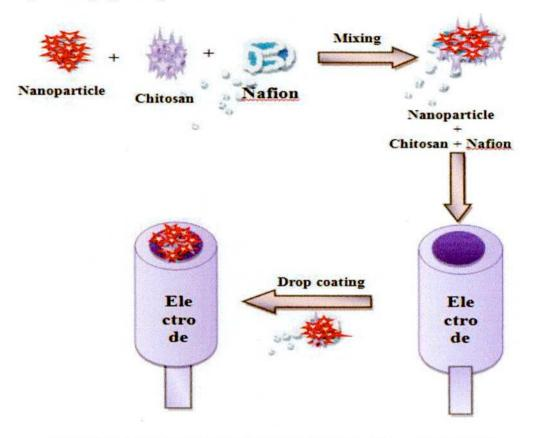
Figure 3.3: A step-by-step diagram of modification of working electrode.
