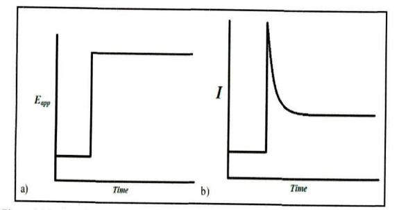
Figure 1.14: a) excitation waveform b) current response output generated from the excitation waveform.
