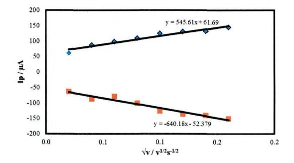
Figure 4.3(b): The anodic and the cathodic peak heights as function of the square root of the scanning rate for PGE.
