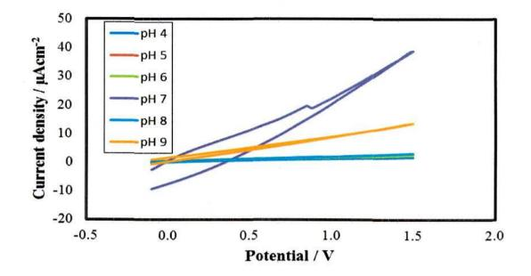
Figure 4.23: CVs of 0.1M PBS 0.05 V/s scan rate at different pH were performed at 2B PDPE.
