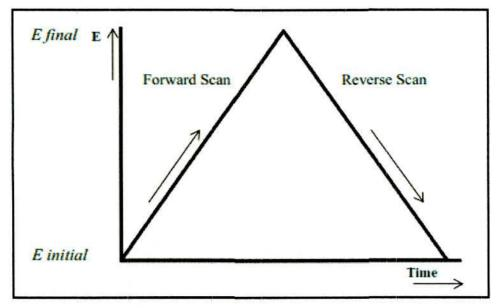
Figure 1.11: Cyclic voltammetry input waveform.
