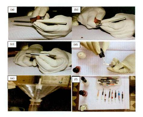
Figure 3.1: Schematic diagram of pencil graphite electrodes fabrication.
