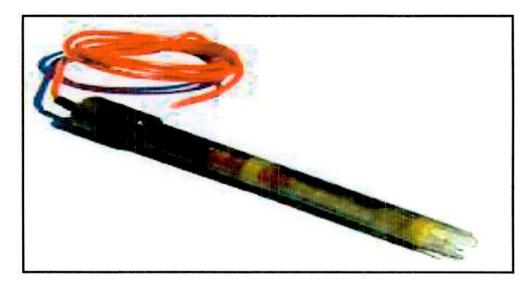
Figure 1.8: Ag/Agcl reference electrode.
