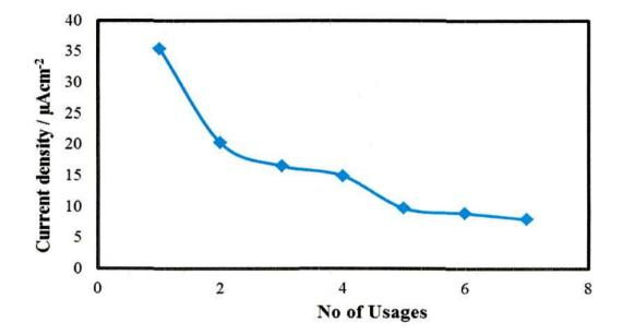
Figure 4.24: Stability of the PDPE over a no. of usages.
