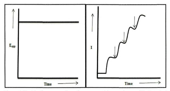
Figure 1.13: (a) Current waveform for amperometric experiments. (b) A typical amperometric plot in stirred solution. Arrows indicate additions of the target analyte.
