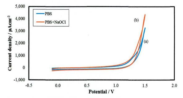
Figure 4.6(a): CVs in 4B PGE (a) in the absence of NaOCl and (b) in the presence of 10 mM NaOCl in 0.1M PBS at  $E_{app}$ = 1.5V (scan rate: 0.05 V/s).
