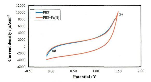
Figure 4.17: CVs in 2B PGE (a) in the absence of  $FeCl_2$  (b) in the presence of Fe in 0.1M PBS containing at  $E_{app}$ = -0.1 to 1.5V (scan rate: 0.05 V/s).
