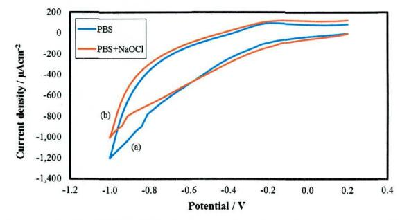
Figure 4.6(b): CVs in 2B PGE (a) in the absence of NaOCl and (b) in the presence of 10 mM NaOCl in 0.1M PBS at E<sub>app</sub>= 0.2 to -1 V (scan rate: 0.05 V/s).
