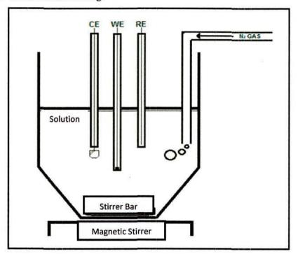
Figure 1.6: Schematic diagram of a voltammetric cell based on a three electrode system. CE: counter electrode, WE: working electrode, RE: reference electrode.
