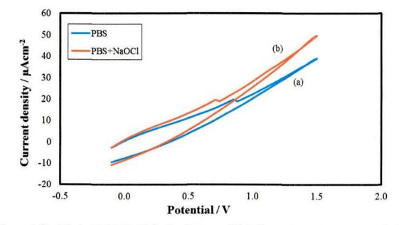
Figure 4.19: CVs in 2B PDPE (a) in the absence of NaOCl and (b) in the presence of 10 mM NaOCl in 0.1M PBS containing at  $E_{app}$ = -0.1 to +1.5V (scan rate: 0.05 V/s).
