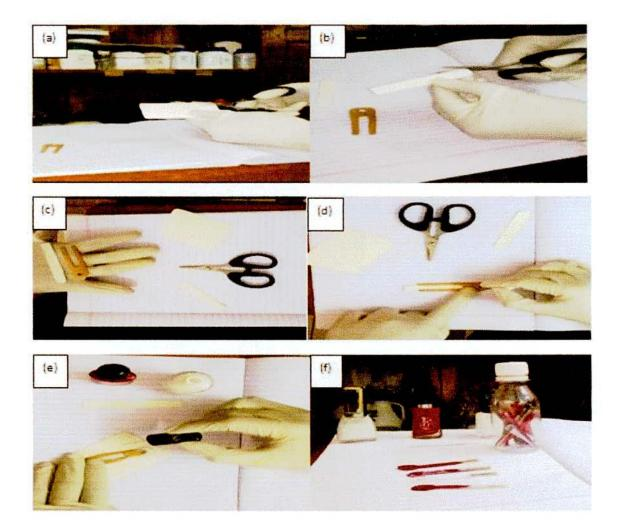
Figure 3.2: Schematic diagram of pencil drawn paper electrodes fabrication.
