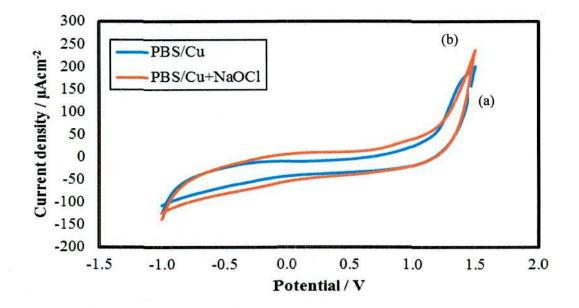
Figure 4.7: CVs of 0.1 M PBS CuO/PGE (a) without NaOCl (b) in the presence of NaOCl at  $E_{app}$ = 1.5 V (scan rate: 0.05 V/s).
