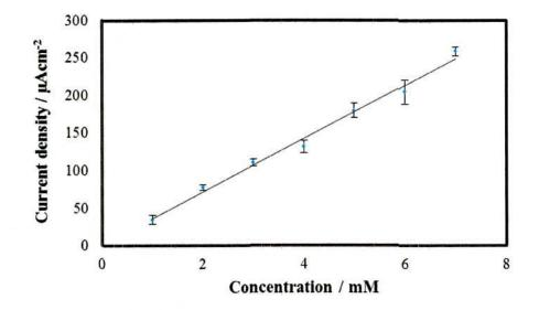
Figure 4.21: The plot of concentration effect current density vs. the corresponding concentrations of NaOCI in PDPE.
