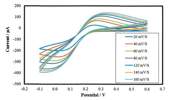
Figure 4.3(a): CVs of Ferricyanide at 2B PGE were performed at concentration of 2 mM of Ferricyanide 0.1 M KNO<sub>3</sub> as supporting electrolyte, different scan rates 20, 40, 60, 80, 100, 120, 140, 160 mV/s.
