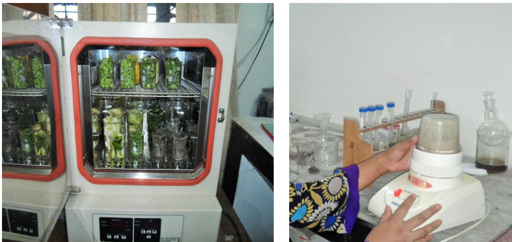
Figure 3.13: Drying and grinding of samples
