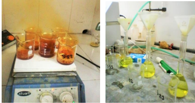
Figure 3.14: Digestion and filtration of samples
