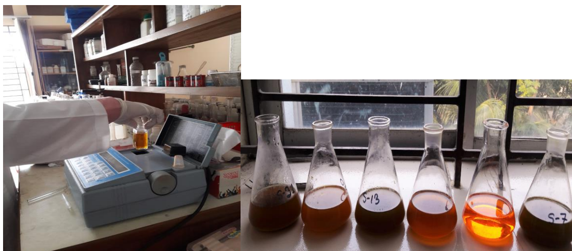
Figure 3.15: Organic matter analysis by UV-VIS Spectrophotometer
