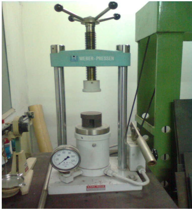
Figure 3.2 Hydraulic press used to make different shaped samples.
