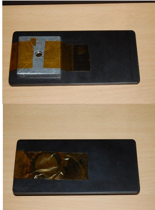
Figure 3.14 Sample preparations for Mössbauer measurement
