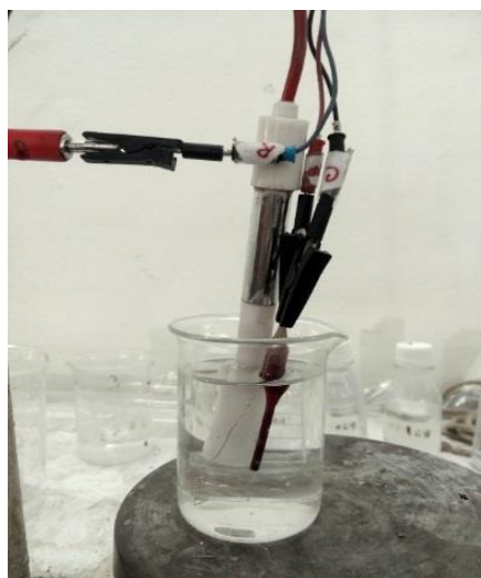
Figure 3.9: Crocodile clips made by stainless steel that is used to connect the electrolytic cell to the potentiometer.
