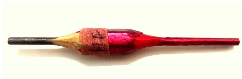
Figure 3.4: HB pencil graphite working electrode used in my research
