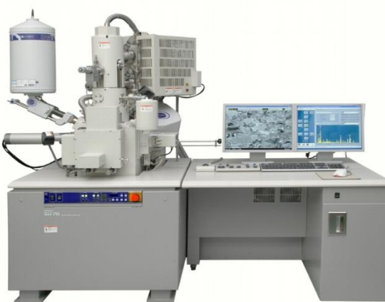
Figure 1.19: A typical SEM instrument, showing the electron column, sample chamber, EDS detector, electronics console, and visual display monitors.
