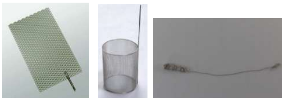
Figure 3.9: (a) Counter electrodes (mesh) (b) Counter electrode used in our research.
