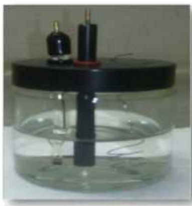
Fig: The three electrode system consisting of a working electrode, a reference electrode and a counter electrode.
