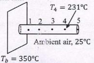
Write down the implicit and explicit finite difference equation of a hot brass plate with the 4(c) 13 following condition shown in figure. Also mention what will be the stability criteria for the explicit method. Assume any time step.
