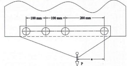
8(b) A plate is lapped over and welded to a gusset plate as shown in figure below. Determine the 19 size of fillet welds to be specified using  $\tau = 140$  MPa through the throats of welds. What maximum value P can be applied vertically if 7 mm welds are used?
