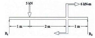
5(b) For the restrained beam shown in figure, compute end moments and maximum  $EI\delta$ .
