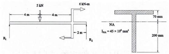
4(b) The T section shown in figure is the cross-section of a beam formed by joining two 18 rectangular pieces of wood together. The beam is subjected to a maximum shearing force of 60 kN. Show that the NA is 34 mm from the top and the  $I_{NA} = 10.57 \times 10^6 \text{ mm}^4$ . Using these values, determine the shearing stress (i) at the neutral axis and (ii) at the junction between the two pieces of wood.
