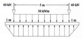
3(b) Draw moment and load diagrams corresponding to the given shear diagram as shown in 17 figure. Specify values at all change of load positions and at all points of zero shears.
