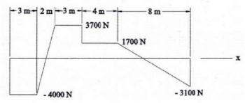
4(a) Determine the maximum tensile and compressive bending stress developed in the beam 17 shown in the figure.
