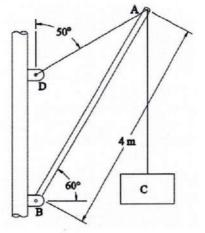
7(b) An aluminum tube of AB of circular cross-section has a guided support at the base and is pinned at the top to a horizontal beam supporting a load Q = 280 kN. Determine the required thickness *t* of the tube if its outside diameter *d* is 180 mm and F.S. = 2.5. Use, E = 75 GPa.
