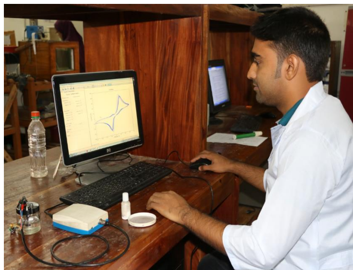
Figure 3.1: Experimental setup (Software controlled Potentiostats ( \mu\text{stat 400} ))
