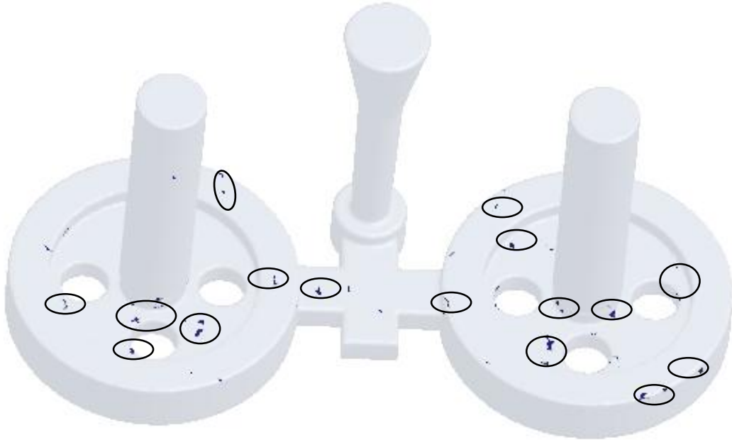
Figure D-2: Air entrapment of cast component in various gating and feeding systems of iteration no.2,4,5, 6, 7 (according to the number declared in table A-1).
