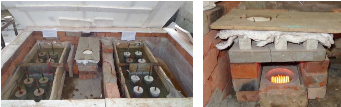
Figure 3.10: Experimental accelerated corrosion test for 45 °C and 60 °C temperatures.
