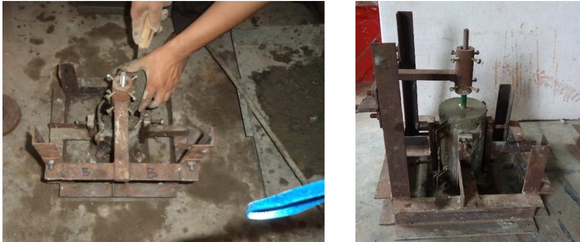
Figure 3.6: Placement of concrete into the mold
