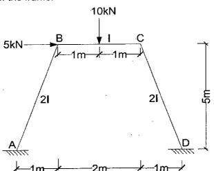
6. Find the forces in the struts and tie rods of the following structure. Diameter of each tie rod is 2cm and each strut is 10cm x 10cm. The beam ABCD is 12cm x 20cm. E for steel is 2 x10<sup>5</sup> N/mm<sup>2</sup> and that for timber is 1x10<sup>4</sup> N/mm<sup>2</sup>.
