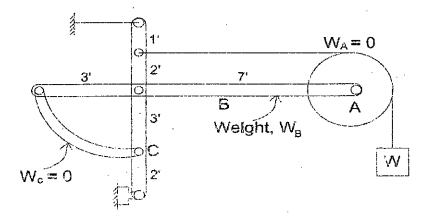
(b) Determine the amount and direction of the smallest force P required to start the wheel in the following figure over the block. What is the reaction at the block?
