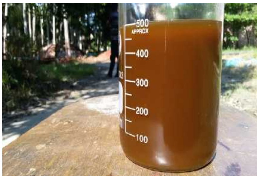
Figure 4.8: Photographic view of Methyl Ester (Biodiesel)
