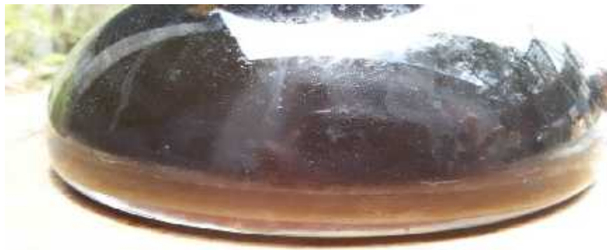
Figure 4.7: Photographic view of biodiesel and glycerol separation
